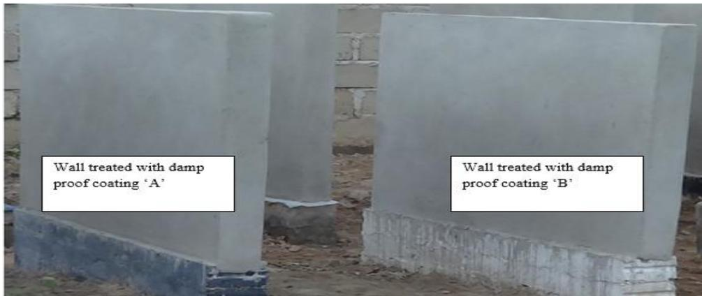
Figure 7. Test walls 4 and 5 after they were treated with the damp proof coatings 'A' (left) and 'B' (right)
