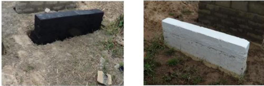
Figure 6 Surface views of test walls after the damp proof coatings 'A' (left) and 'B' (right) were applied
