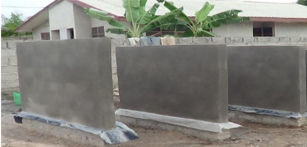
Figure 4. Test Walls after the DPCs were laid
