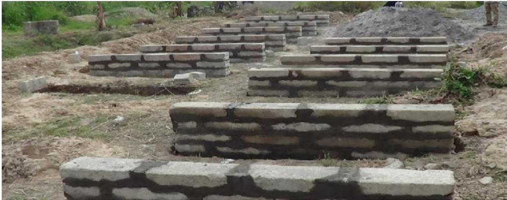
Figure 2. Erected Test Walls- Test walls from SBs are on the extreme left while those from the CBs are on the extreme right.
