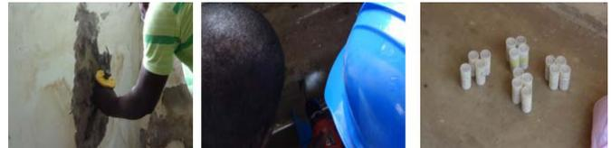
**Figure 5.** Mortar sampled and placed in 35 mm camera film cases
