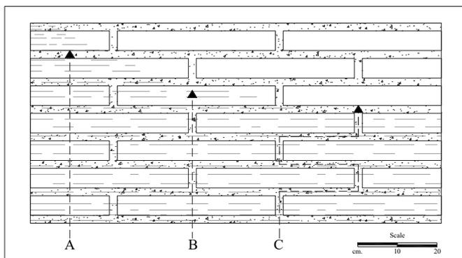
**Figure 2.** Possible routes of moisture in a masonry wall (Massari and Massari 1993)
