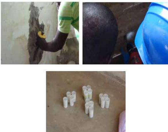
Figure 9. Sampling of mortar
