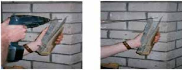
Figure 4. Drilling of brick samples from an affected wall
