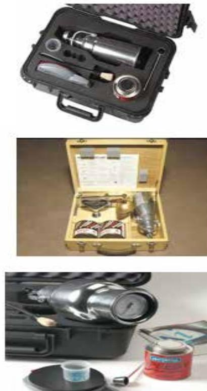
Figure 2. Calcium Carbide meter/ speedy tester used to measure moisture contents of samples
