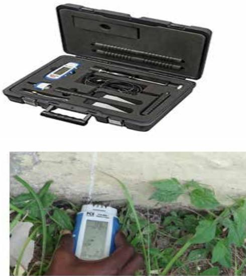
Figure 7. PCE-MMK1 Moisture meter kit used in the study
